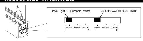
Open the end cap the side with AC wire as the picture shows. Moving the Dip to choose the CCT or you want as the label shows.
