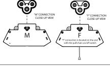
"F" Connection, end with the Pull-chain on/off switch.
